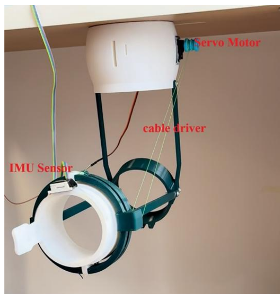
Figure 4 – Experimental setup for controlling pronation/supination movement at the elbow joint: prototype equipped with servo motor, cable driver, and IMU sensor
